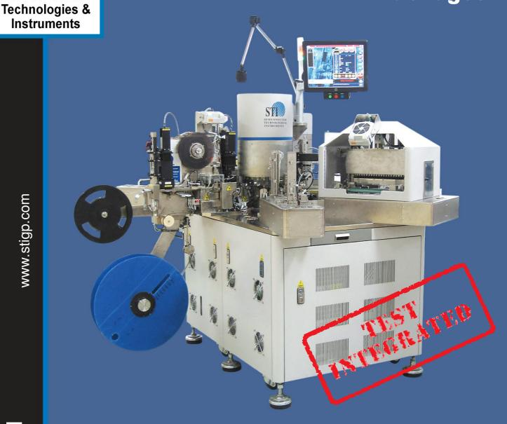
The AT468 is a high speed multi-function scan-pack handler engineered for Lead and Leadless packages. This fully automated design consists of a primary 24-station rotary turret coupled with a secondary multi-station inspection table.
